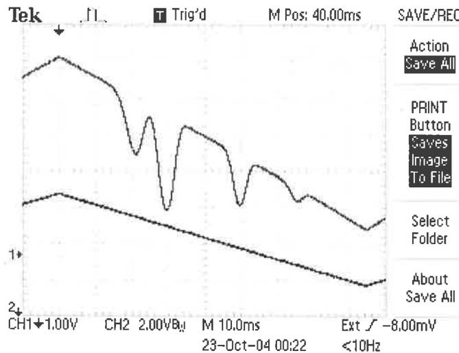
Figure 11: Expanded Scan Showing Four Absorption Lines
