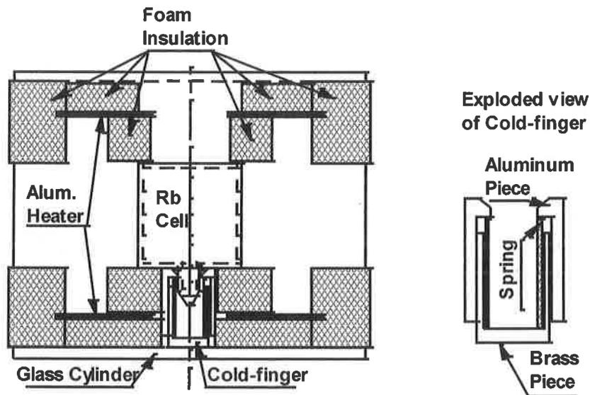
Figure 17: Cross section of Cell Heater Assembly
