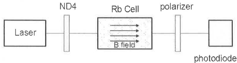
Figure 1. Basic optical layout. The large ND filter makes sure one is in the unsaturated regime. The light coming out of the laser is linearly polarized, so only one polarizer is needed.
