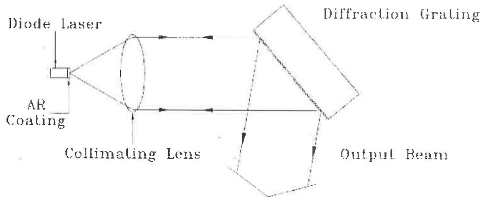
Figure 4: Basic configuration of the diode laser system
