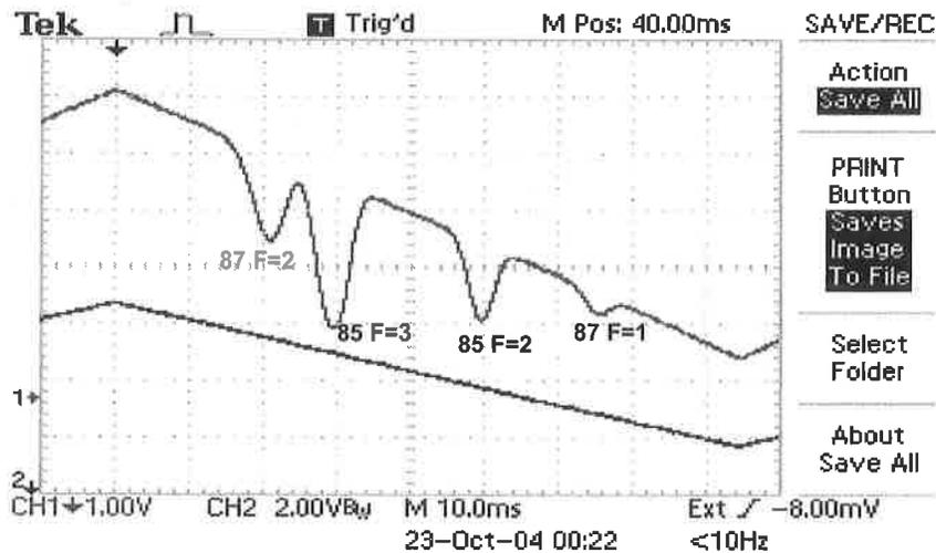
Lower Trace: Sawtooth ramp voltage which is creating a “sweep” of both the laser current and the grating angle. This, in turn, creates the change in the laser frequency. Falling sawtooth indicates increasing frequency.
