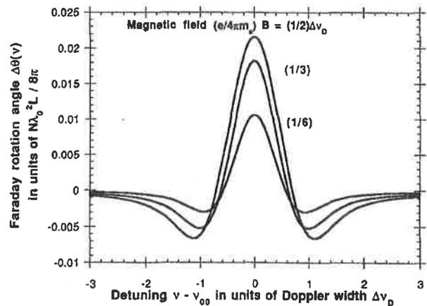
Fig. 5. Faraday rotation angles computed for the model problem of this paper, in the presence of Doppler broadening, for three values of magnetic field strength  $B$ :  $(e/4\pi m_e) B = \Delta\nu_D/6$ ,  $\Delta\nu_D/3$ , and  $\Delta\nu_D/2$ .
