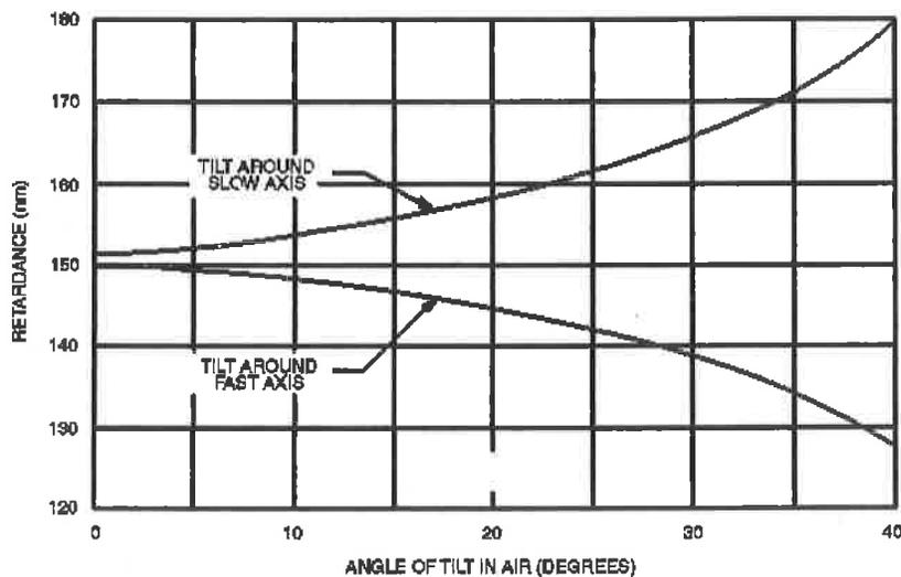
Figure 20: Tilt Tuning of Quarter Wave Plate
