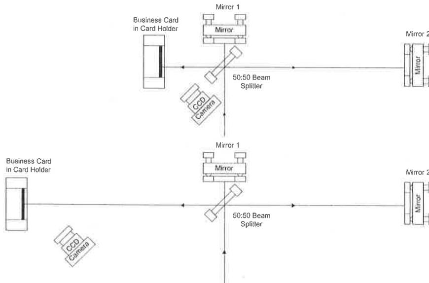
Figure 3 Iterative procedure to get two beam co-linear.
