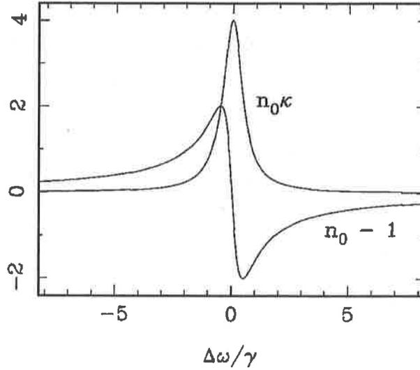
Figure 3. Plot of the absorption  $n_0\kappa$  and refractive index change  $n_0 - 1$  for a gas near an atomic resonance. Note the index change is proportional to the first derivative of the absorption.
