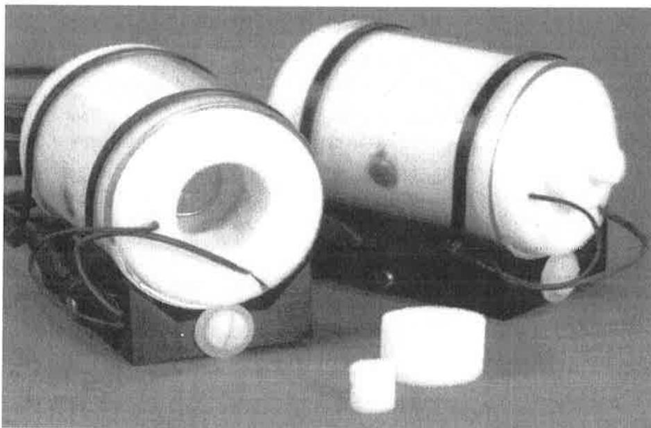
**Figure 21: Cell assembly showing placement of foam plugs**
