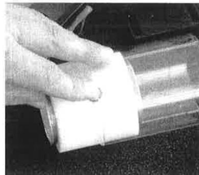
Figure 18: Insertion of Cold-finger into Cell Assembly
