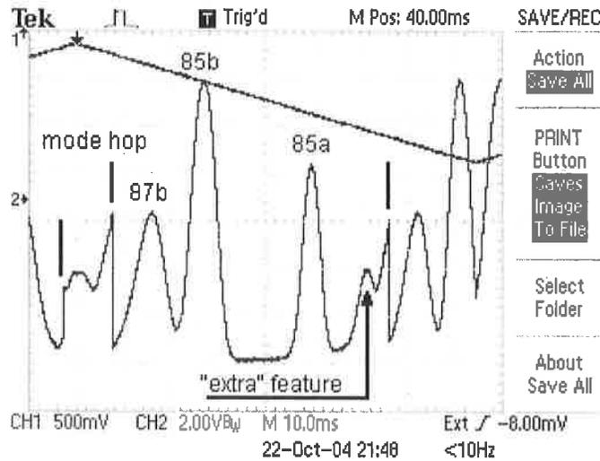
Figure 9: Scan showing first three absorption lines
