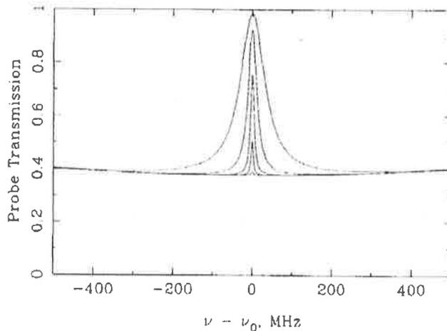
Figure 6. Calculated saturated-absorption spectra for two-level atoms, for  $(\tau, I/I_{sat}) = (1,0.1), (1,1), (1,10), (1,100),$  and  $(1,1000)$ . Note at large laser intensities the saturated absorption feature is “power broadened” as the line saturates.
