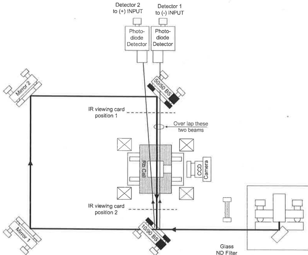
Figure 4. Aligning pump and probe beams.
