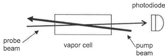
Figure 1: The basic saturated absorption spectroscopy set-up.
