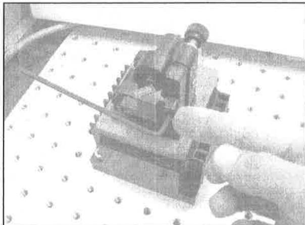
**Figure 11: Initial installation of the Grating:
