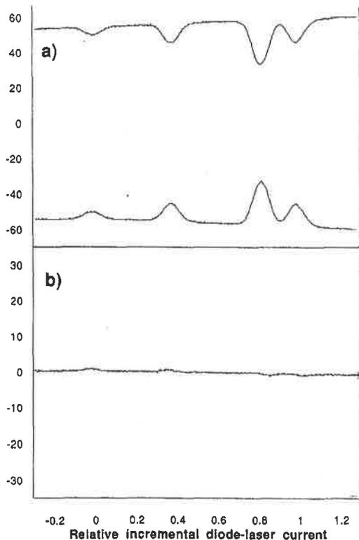
Fig. 8. (a) The signals obtained from the two photodetectors of the polarization analyzer of Fig. 6, under conditions of polarizer angle  $\phi=45^\circ$ , zero magnetic field, and one signal electronically inverted. (b) The sum of the two signals of (a), further expanded vertically by a factor of 2; this is the signal representing zero Faraday rotation.
