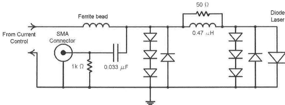
**Figure 6: Schematic High Frequency Modulation Circuit.** Also shown are two sets of protection diodes. The three diodes in series are 1N4148's and the diodes used to prevent reverse voltages are 1N5711's.
