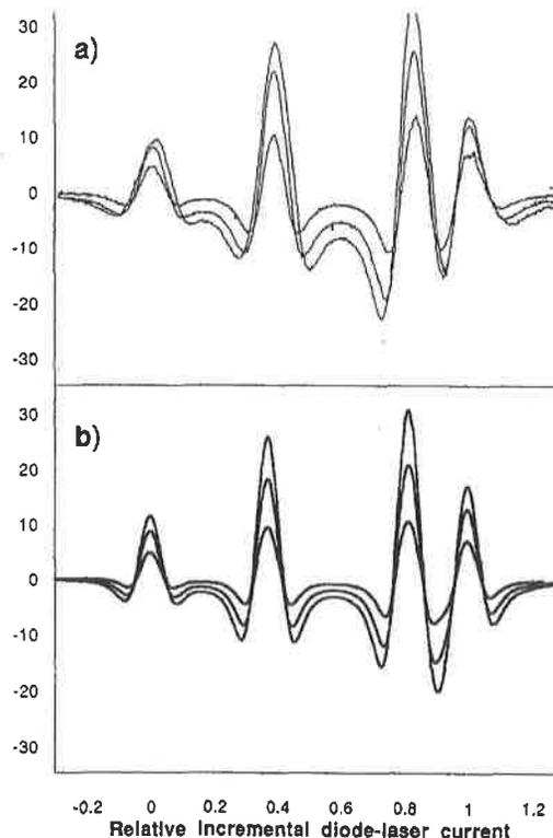
Fig. 9. (a) The experimental Faraday-rotation signal for three values of magnetic field strength ( $B=5$ , 10, and 15 mT), obtained at the same scale as the "baseline" data of Fig. 8(b). (b) Theoretical Faraday-rotation signals expected for this experimental situation, computed using the model described in the text. The theory uses the same horizontal and vertical scaling as in Fig. 7(b), and no adjustable parameters.
