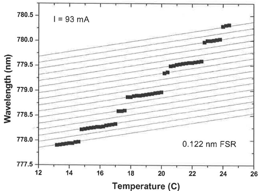
**Figure 6:** Output wavelength of a free-running (*i.e.* no external optical feedback) Sanyo DL-7140-200S diode laser as a function of diode temperature. (The behavior of other diode lasers is similar.)
