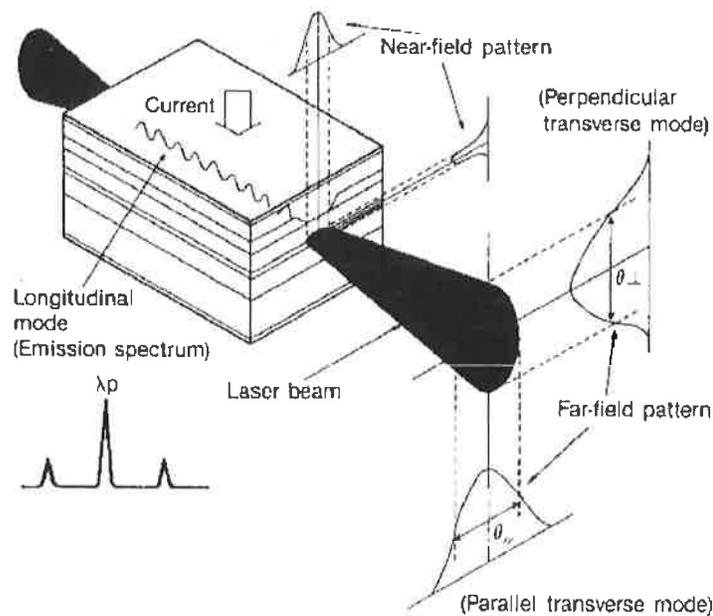
**Figure 2:** Schematic view of a laser diode chip
