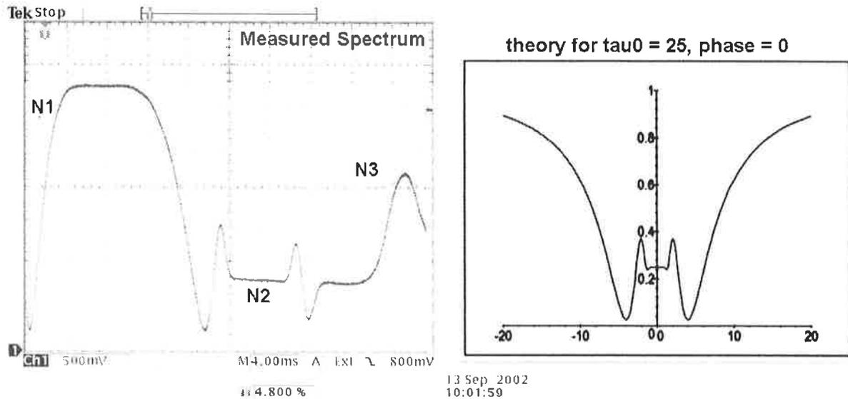
Figure 5. A comparison of a measured spectrum (left) with a calculated spectrum (right). The plot shows  $I(\Delta\omega)/I_0$  versus  $\Delta\omega/\gamma$ . The calculation assumed  $\tau = 25$  at line center and  $k\Delta L = 0$ . The measured spectrum is for the 85b line, but the adjacent 87b line complicates the right side of the spectrum (marked by N3). The center of the 85b line is at N2. The feature at N1 is an artifact of the laser scanning.
