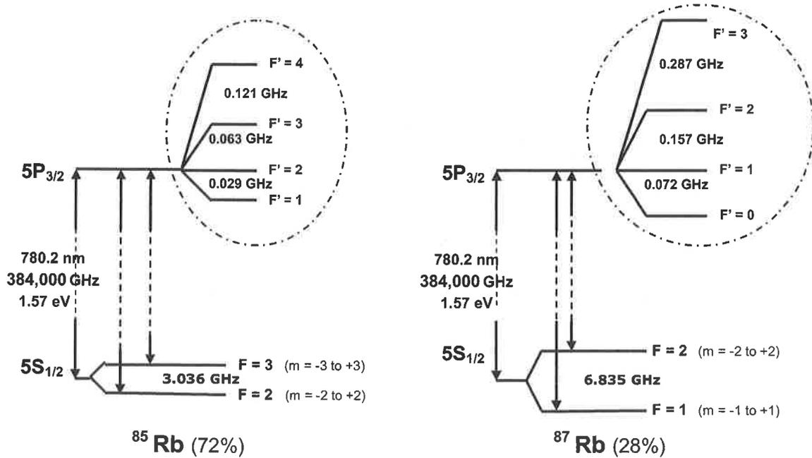
Energy Diagram shows D2 transitions only. The D1 transitions at 794.8 nm are not shown
