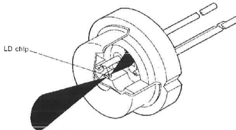
**Figure 1:** Cut-away view of a typical laser diode can, like those used in the TeachSpin laser
