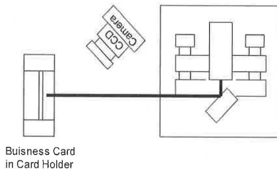
**Figure 9: Setup for Viewing Beam Profile and Retro-reflection.**
