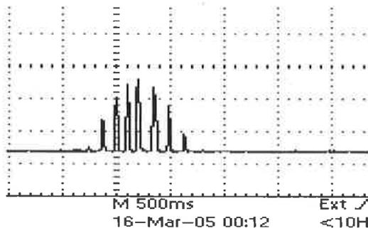
Figure 3, at the right, shows an oscilloscope trace of the intensity of the laser as the TOP knob is adjusted. It will give you an idea of how the brightness of the spots you are seeing is varying. It is hard to tell the middle ones apart. For best alignment leave the laser in the middle of this vertical mode pattern as best you can. It is not necessary to sit right on one of the mode maxima, but only near the center of the mode pattern. The correct mode
