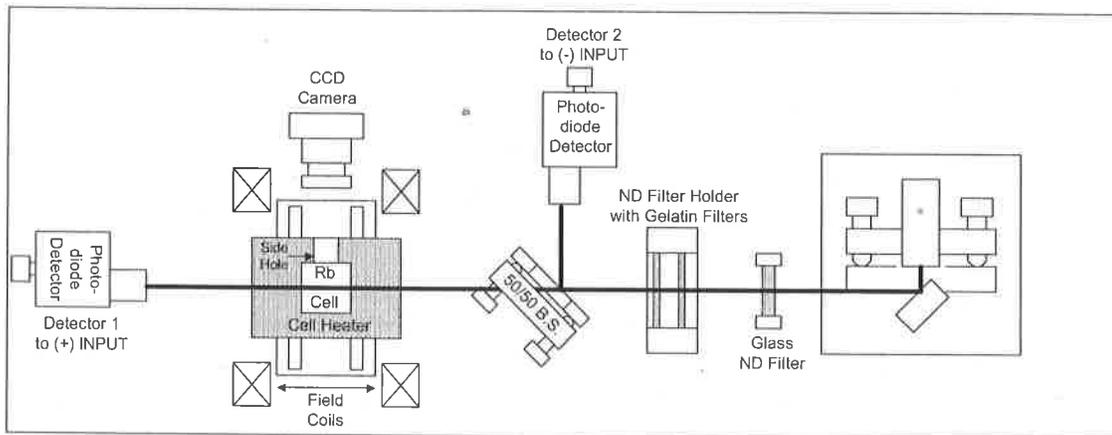
Figure 12: Apparatus set up to use two detectors
