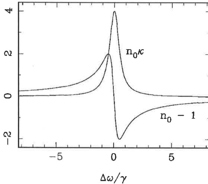
Figure 1. Plot of the absorption  $n_0\kappa$  and refractive index change  $n_0 - 1$  for a gas near an atomic resonance. Note the index change is proportional to the first derivative of the absorption.
