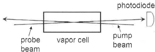
Figure 1. The basic saturated absorption spectroscopy set-up.
