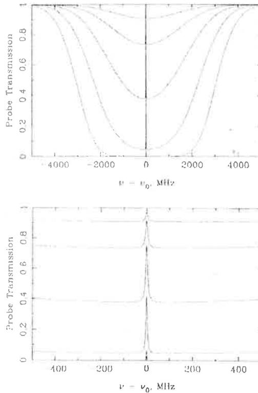
Figure 5. Calculated saturated-absorption spectra for two-level atoms, for  $(\tau, I/I_{sat}) = (0.1, 10)$ ,  $(0.316, 10)$ ,  $(1, 10)$ ,  $(3.16, 10)$ , and  $(10, 10)$ . The two plots show the same spectra with the frequency axis at different scales. Note the overall Doppler-broadened absorption, with the small saturated-absorption feature at line center.
