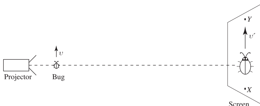
Figure 12.4: The shadow of the bug moves across the screen at a velocity v' greater than c , provided the screen is far enough away.
